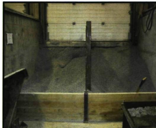
Figure 3.13 – Pierre calcaire 5-14 mm
