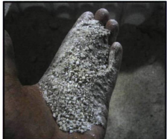
**Figure 3.17 – Sable calcaire
