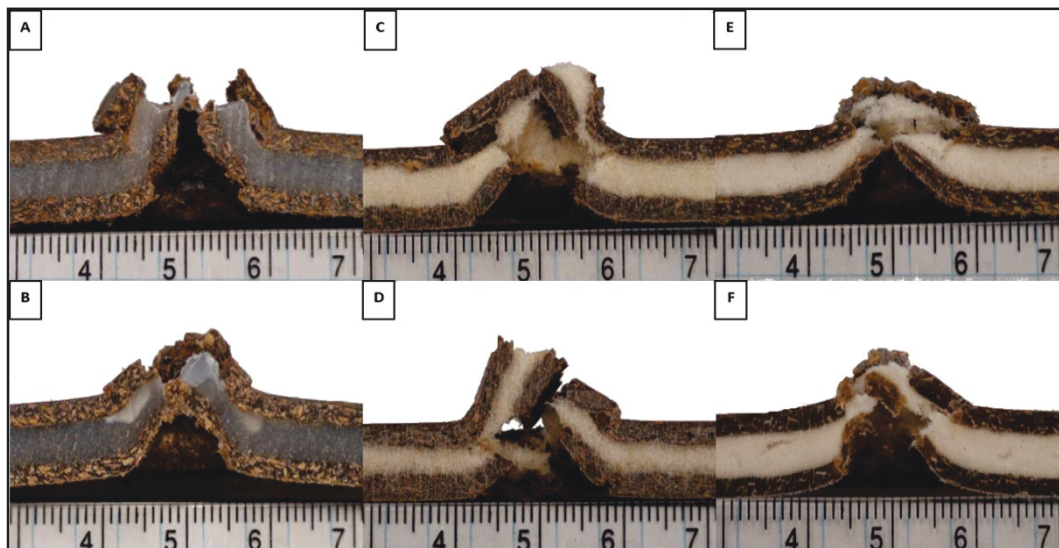
Figure 4.8. Cross-section images of the perforated sandwich structures: A) 40(1)-0-40(2), B) 10(1)-0-20(2), C) 40(1)-0.6-40(2), D) 10(1)-0.6-20(2), E) 40(1)-1.2-40(2), and F) 10(1)-1.2-20(2).
