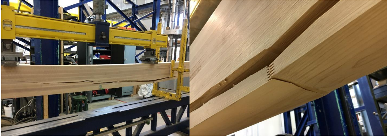
Figure 22. Failure of a yellow birch glulam beam initiated at a finger joint.
