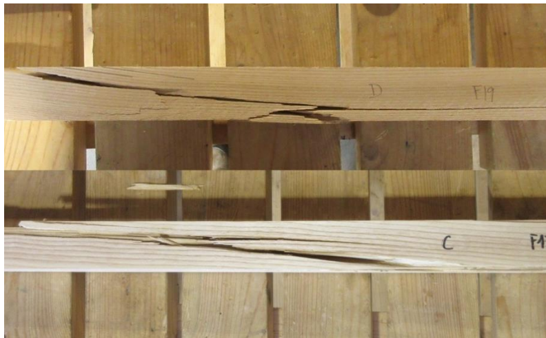
Figure 9. Failure pattern following the ring boundaries on radially sawn white ash specimens.
