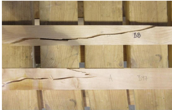
Figure 8. Wavy grained yellow birch specimens after failure.
