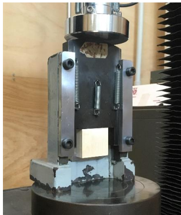
Figure 12. Block shear testing device.
