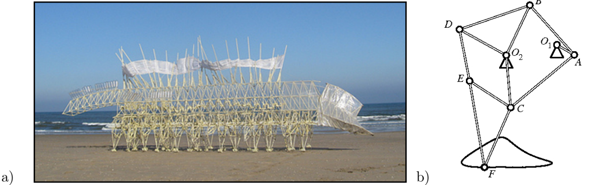
Figure 2.5: a) The Strandbeest is a kinematic sculpture by Theo Jansen [24]; b) The legs [51] are eight-bar linkages which yield organic-looking walking motion.
