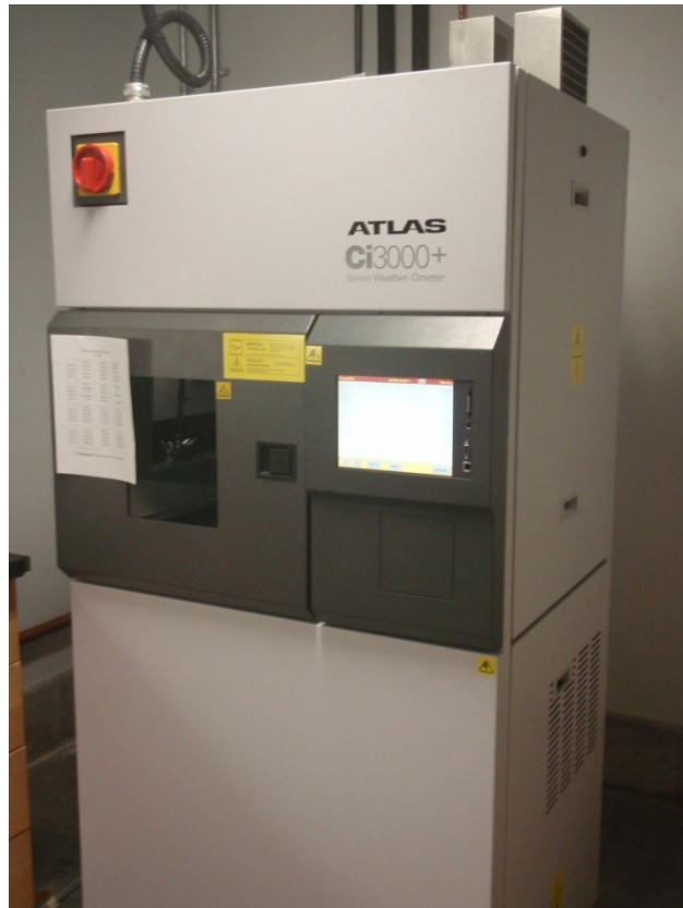
Figure A.17. An example of an accelerated UV aging system (Atlas Inc., USA).
