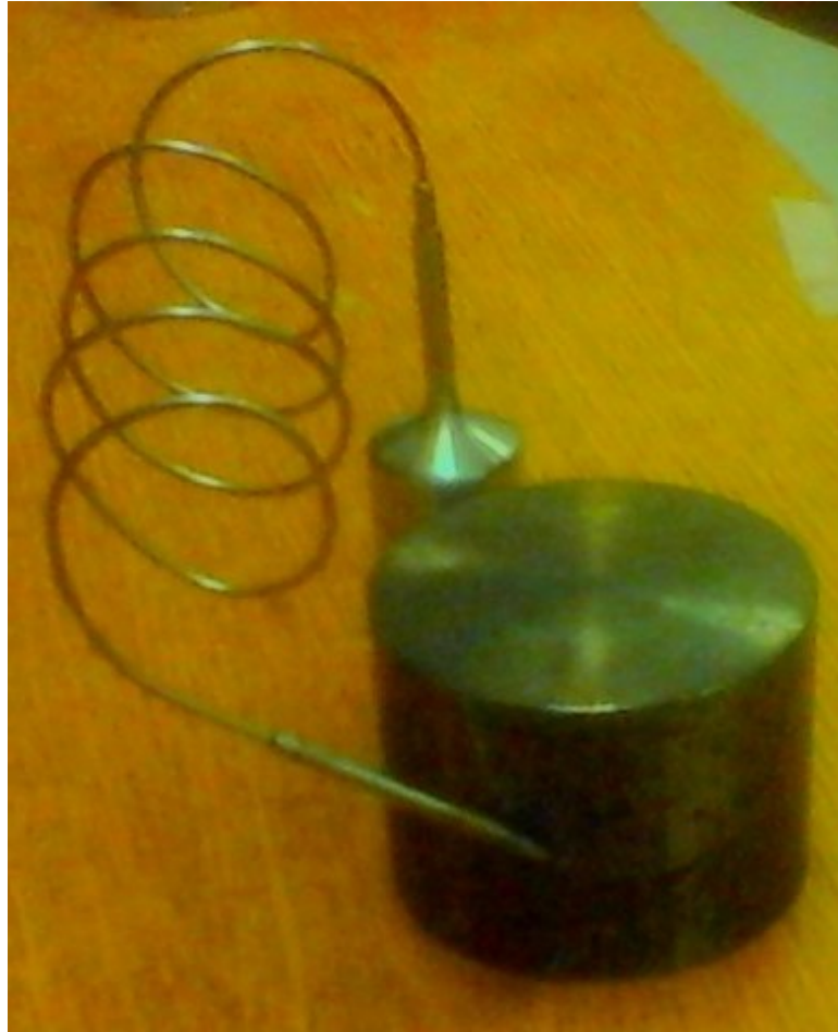
Figure 6-5. Steel cylinder and thermocouple.
