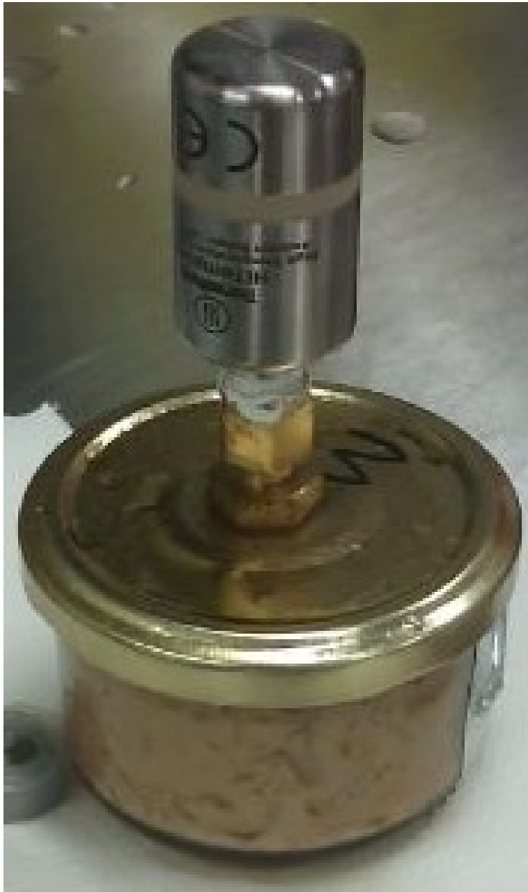
Figure 6-2. Glass jar filled up with foie gras emulsion having a thermocouple to measure the temperature at the center.
