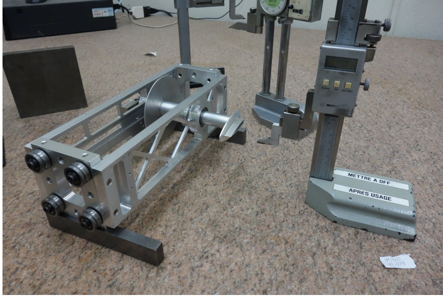
Figure A.3: Assembly of the blade with respect to the pitch holder in order to obtain a pitch angle of 0^\circ when the pitch holder is used.
