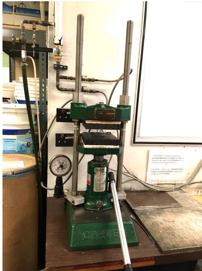
Figure 4.6. Manual press with heating plates to press the samples for the rheometer
