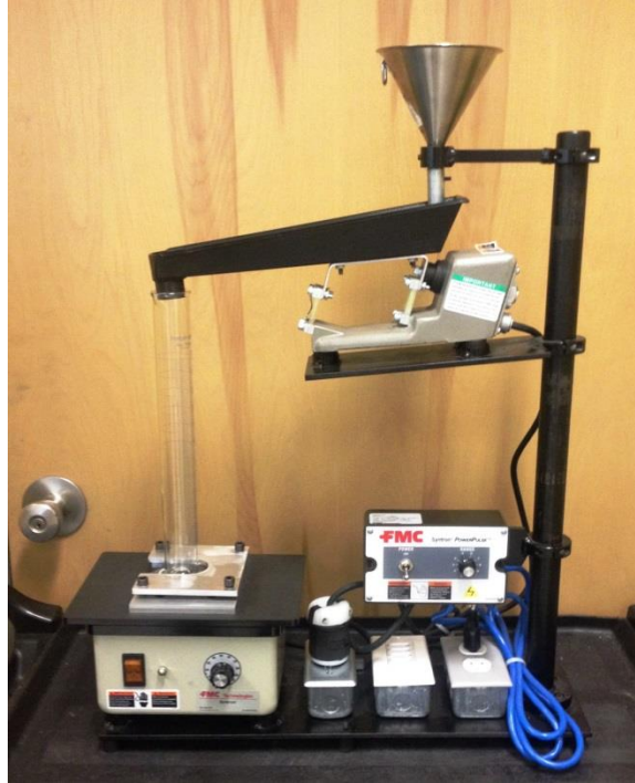
Figure 4.2. Vibrated Bulk Density (VBD) test set up
