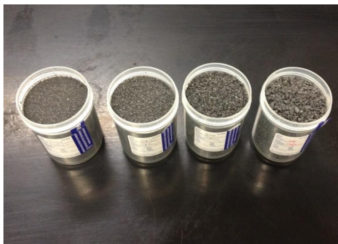
Figure 4.1. Crushed and sieved coke particles. From right to left: -4+8 mesh, -8+14 mesh, -14+30 mesh, -30+50 mesh
