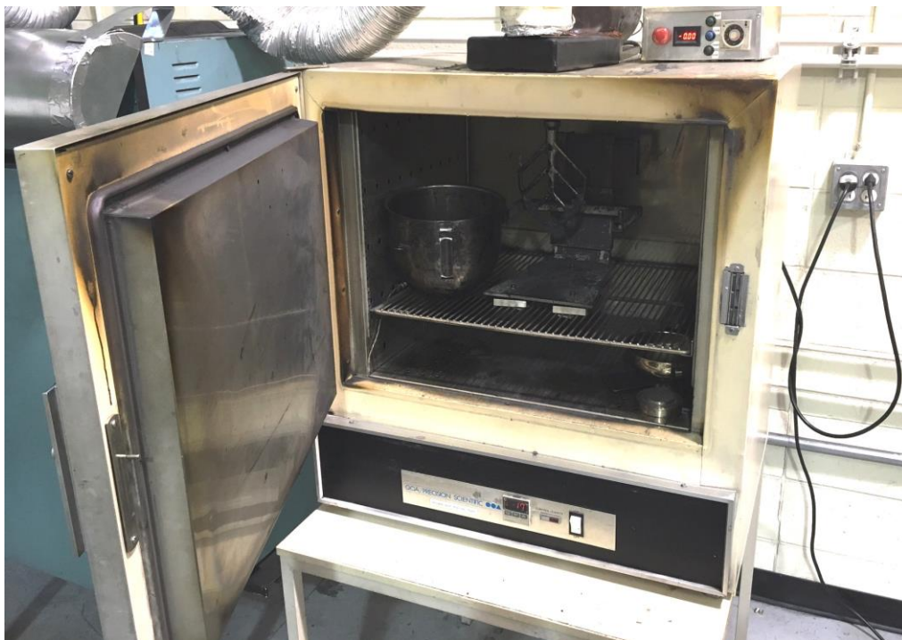
Figure 4.4. . High temperature mixer used to prepare coke and pitch mixtures
