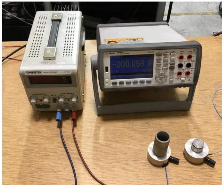
Figure 4.9. The set-up to measure the electrical resistivity of coke powders; sample holder, multi-meter and the DC current source
