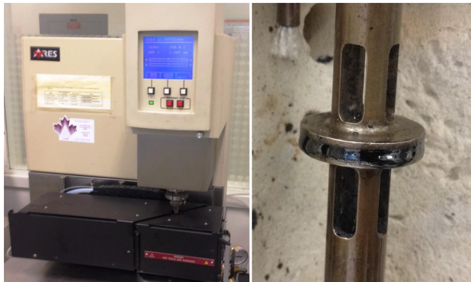
Figure 4.7. Dynamic Shear Rheometer (right) and a pitch sample being tested (left). The black part in the DSR instrument is the sample bath which keeps the temperature constant during the test.
