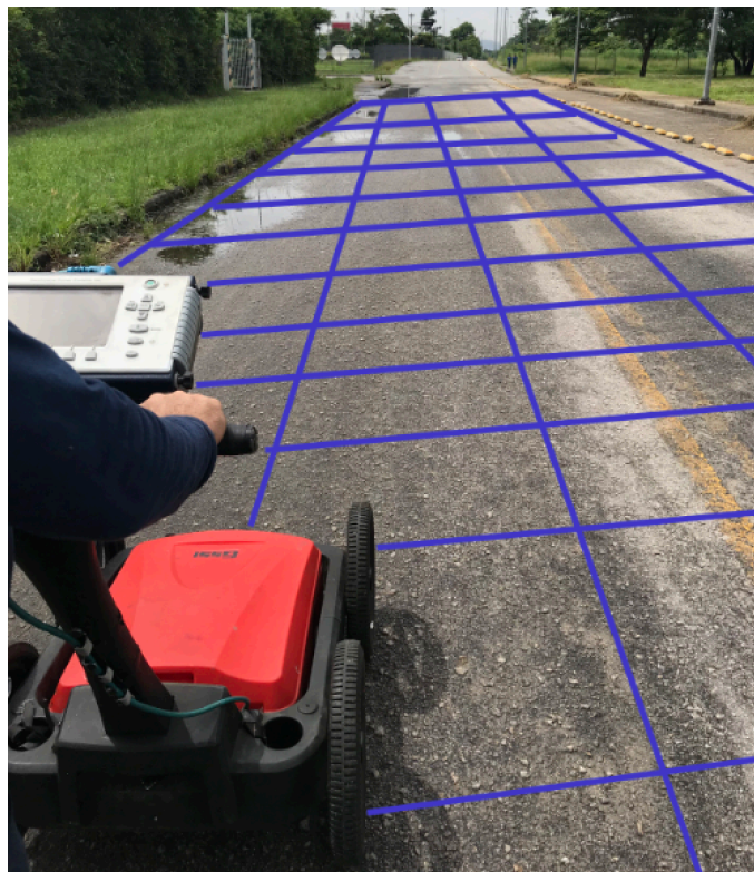
Figure 4.8: GPR survey in progress using a GSSi 3000 (100 MHz antennas) along a street located at the Federal University of Rio de Janeiro (Brazil). A fictive survey mesh is overlaid on the photograph to illustrate the survey strategy.
