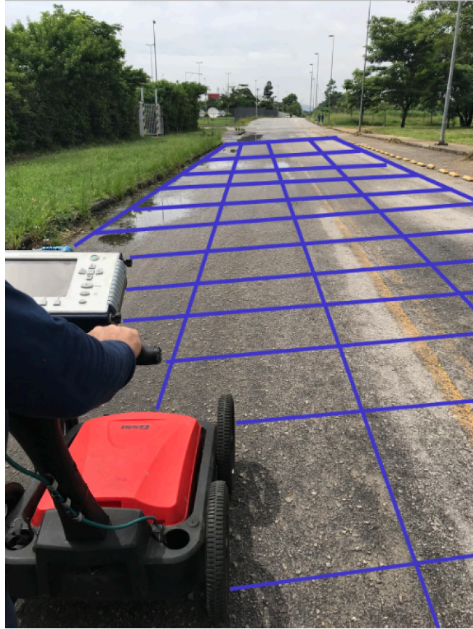
Figure 1.3: A fictitious GPR mesh showing the line pattern followed by a GPR operator.
