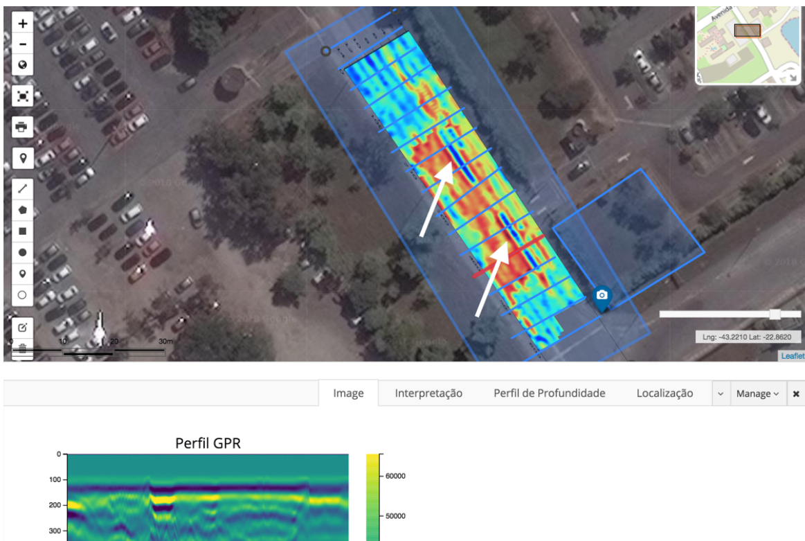
Figure 5.7: GPR depth slice (top figure) showing the likely existence of a water main (identified by white arrows) and radargram (bottom figure).
