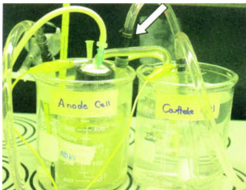
Figure 1.8. Variations on two-chamber reactors. A salt bridge-type MFC used by Min et al. (2005a) between the chambers (arrow), but the system had high internal resistance resulting in low power densities. 77
