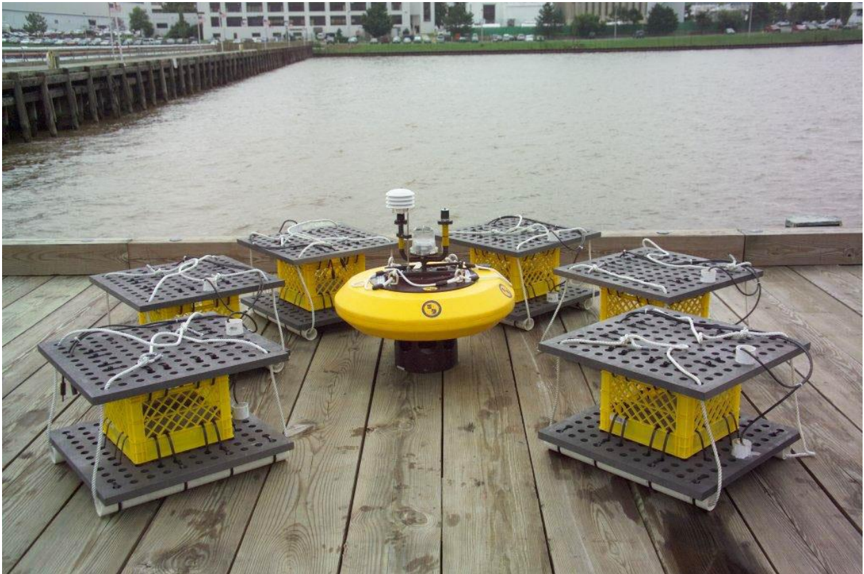
Figure 1.9. A real benthic microbial fuel cell. 83,84
