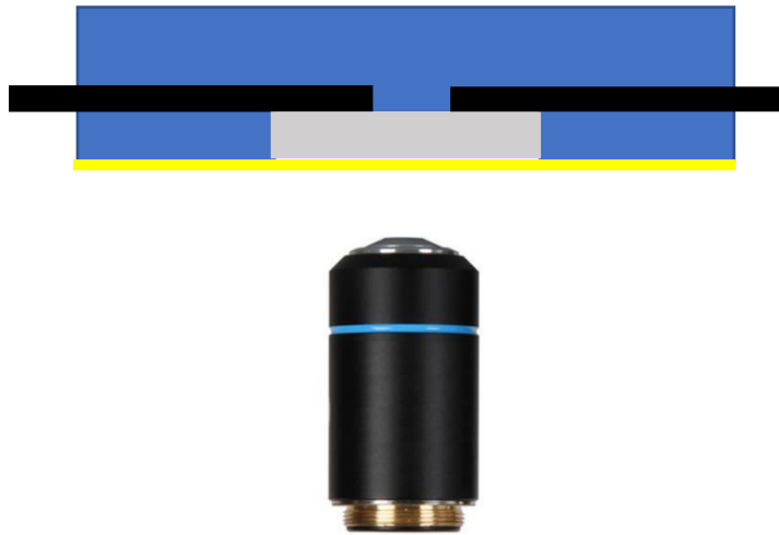
Figure 6.1. Microfluidic MFC device with two graphite electrodes for non-destructive real-time imaging. A channel 160 \mu\text{m} deep and 12 mm wide covered by a glass cover slip allows imaging with confocal scanning laser microscopy.
