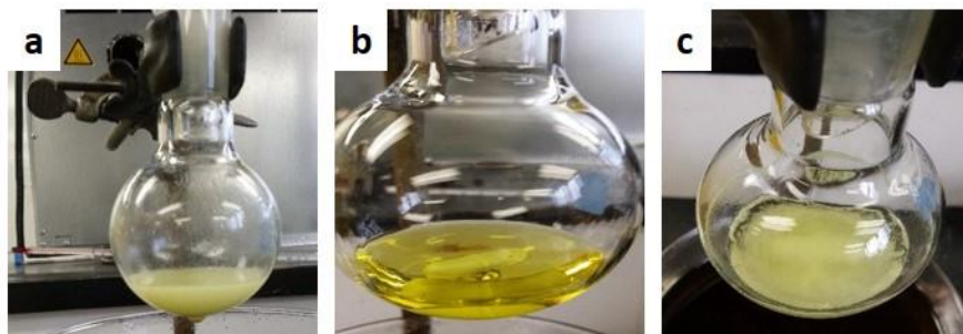
Figure S7.1. Time-lapse views of the reaction mixture in the presence of MO-CTAB1:3 catalyst: (a) beginning of the reaction, (b) during the reaction, and (c) end of the reaction.
