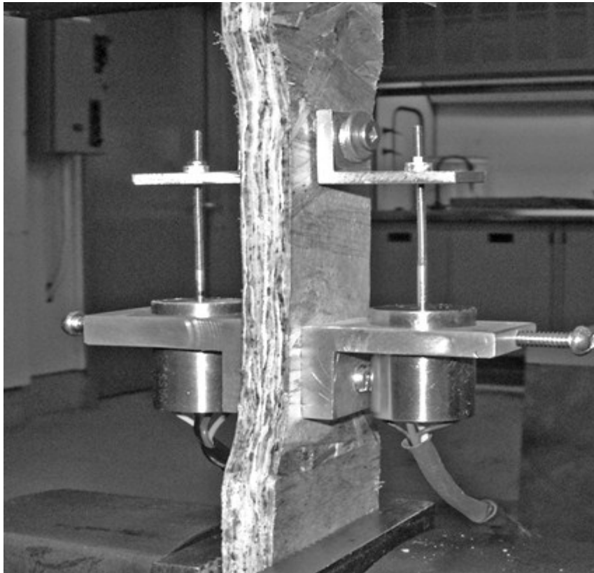
Figure 3.3. — ASTM D1037 in-plane tension test setup with two DCDTs.
