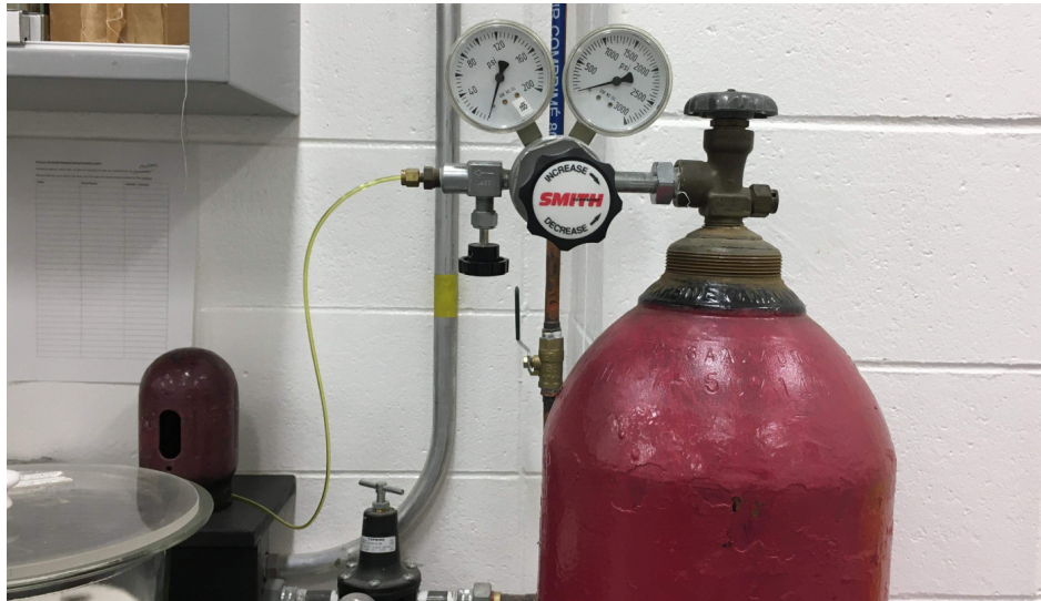
Figure 4.5: Nitrogen gas cylinder and its two-gauge regulator
