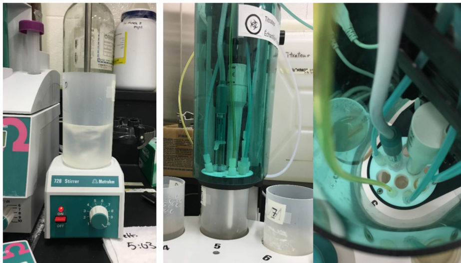
Figure 4.6: From left to right: sample mixing with a magnetic mixer, sample processor from the front with the yellow gas tube installed on its head, sample processor from the top view
