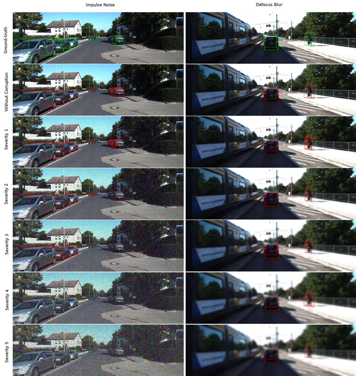
FIGURE A.6 – Ground truth and detection results for two samples from the KITTI-C dataset for impulse noise and defocus blur corruptions. From top to bottom : ground truth, without corruption, and corruption with severity 1 to 5.
