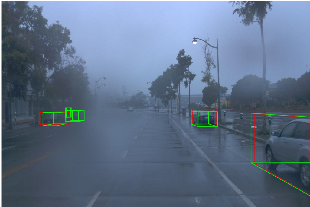
FIGURE 3.7 – Ground truth and detection results for samples from Waymo-Rainy. Green bounding boxes represent the ground truth, and the red bounding boxes represent the detection results.
