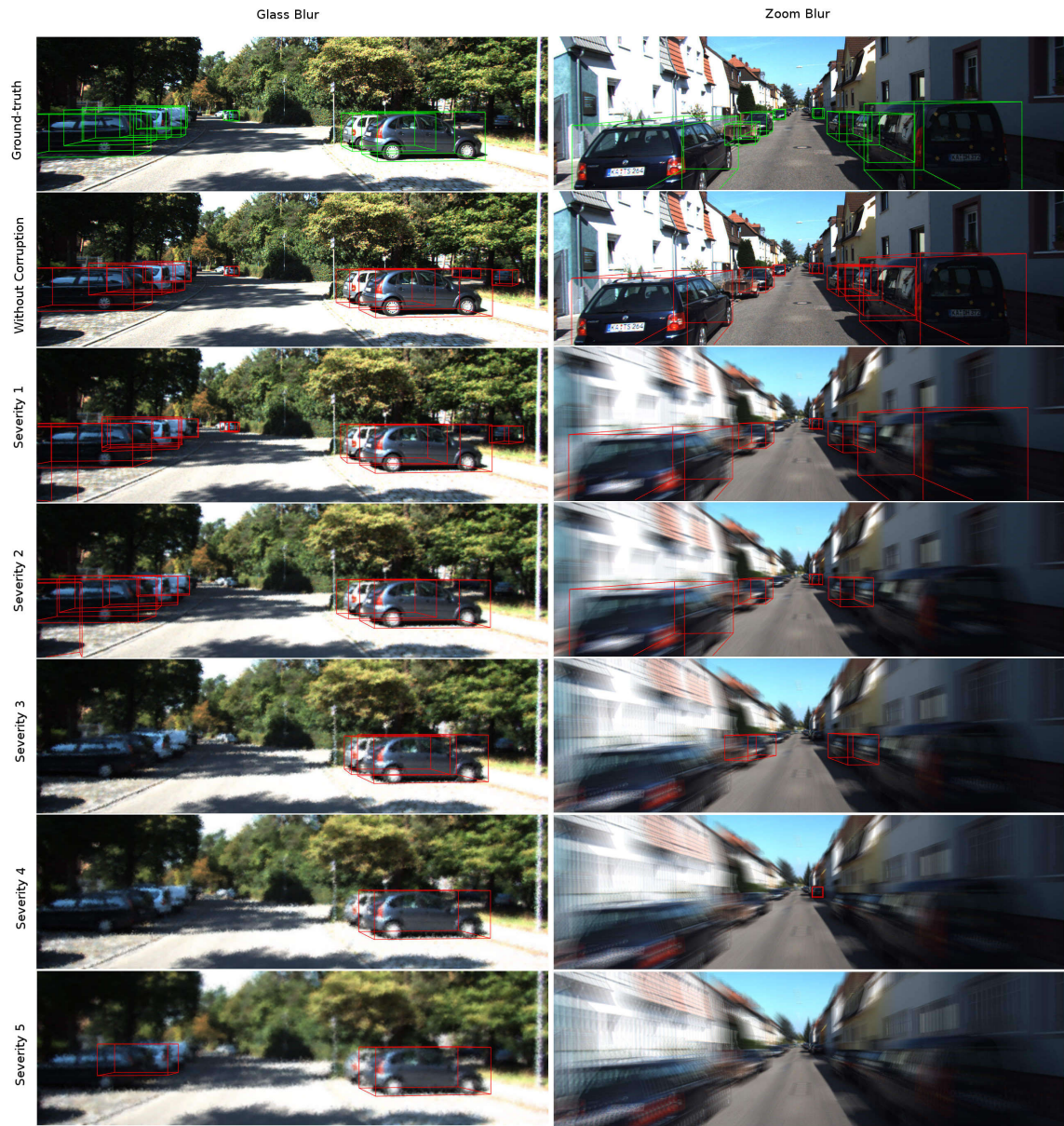
FIGURE A.4 – Ground truth and detection results for two samples from the KITTI-C dataset for glass blur and zoom blur corruptions. From top to bottom : ground truth, without corruption, and corruption with severity 1 to 5.
