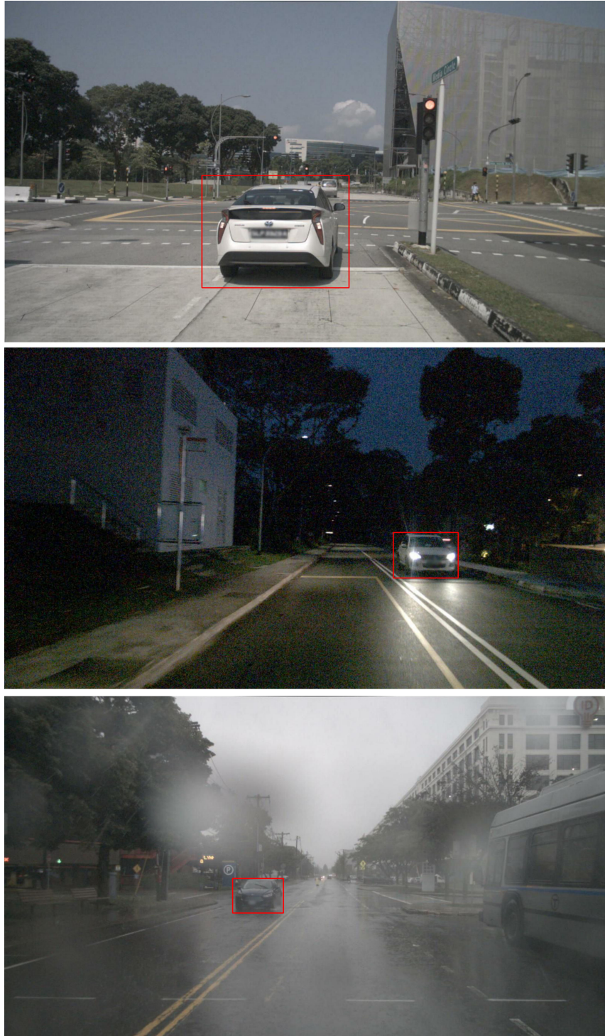
FIGURE 2.2 – Visualization of the ground truth 2D bounding boxes for three sample images in clear, night, and rain from the nuScenes dataset [5]. Red bounding boxes correspond to the car object class ground truth.
