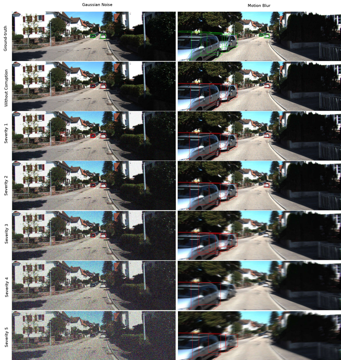
FIGURE A.3 – Ground truth and detection results for two samples from the KITTI-C dataset for Gaussian noise and motion blur corruptions. From top to bottom : ground truth, without corruption, and corruption with severity 1 to 5.
