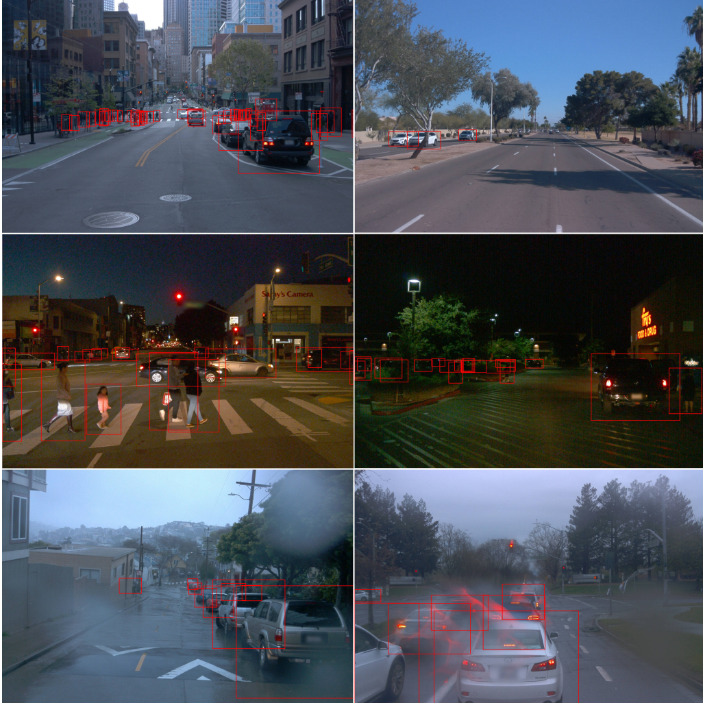
FIGURE 2.3 – Visualization of six sample images with their ground truth 2D bounding boxes in diverse weather and lighting conditions from the Waymo dataset [1].
