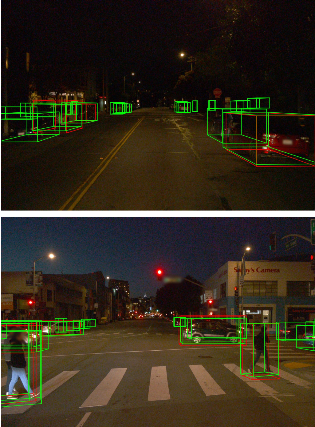
FIGURE 3.8 – Ground truth and detection results for samples from Waymo-Night. Green bounding boxes represent the ground truth, and the red bounding boxes represent the detection results.
