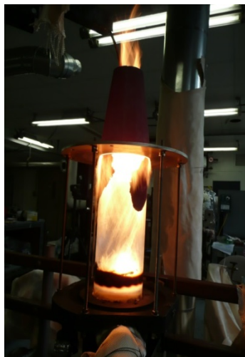
Figure 76 Soot formation during the combustion of the B20 blend at ( \phi = 1 )
