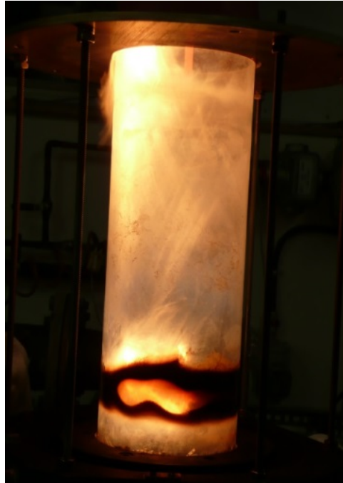
Figure 77 Soot formation during the combustion of the B20 blend at ( \phi = 0.8 )
