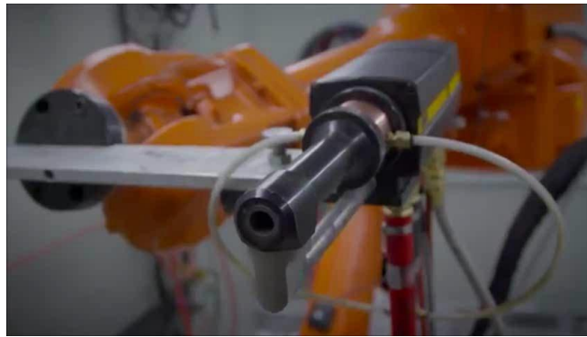
Fig. 19. HVOF gun that applied the coating
