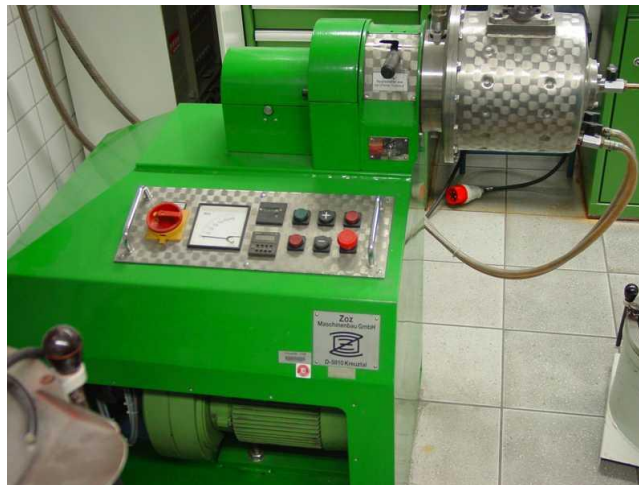
Fig. 18. High energy ball milling apparatus
