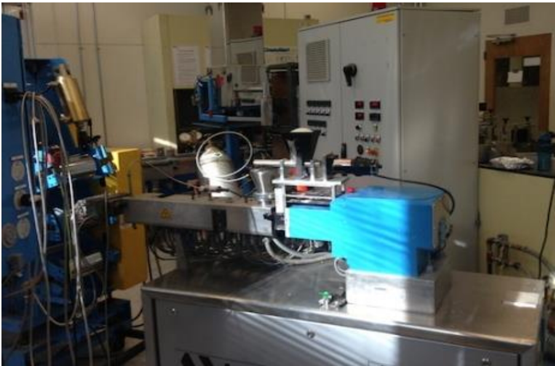
Figure 0.1. Extruder equipped with a flat die to produce film/sheet.
