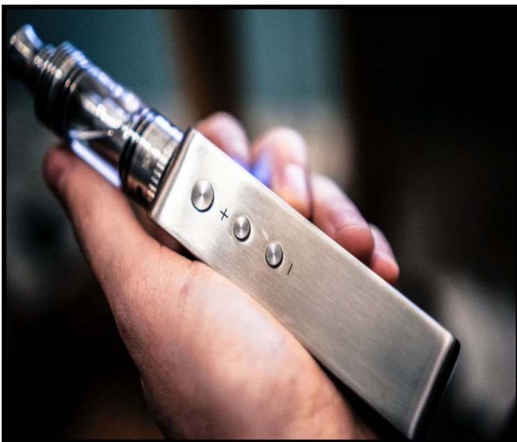
Figure1.15: Fourth generation of e-cigarette. This is the biggest e-cig in term of size and battery capacity. It consists of an advanced personal vaporizers with a fat tube shape, a replaceable battery that give the chance to control voltage, and large reservoir for e-liquid storage. This figure is adapted from https://eciglopedia.com/the-4-generations-of-electronic-cigarettes/
