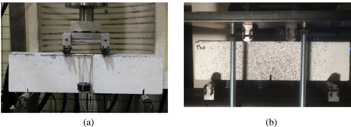
Figure 6.3. Test set-up for (a) static test for pre-cracking; (b) Sustained loading test setup. As for the 3 rd stage, a steel frame apparatus was built to load the samples with dead weight by means of lever arms Figure 6.4b. The loading history is illustrated in Figure 6.4a.
