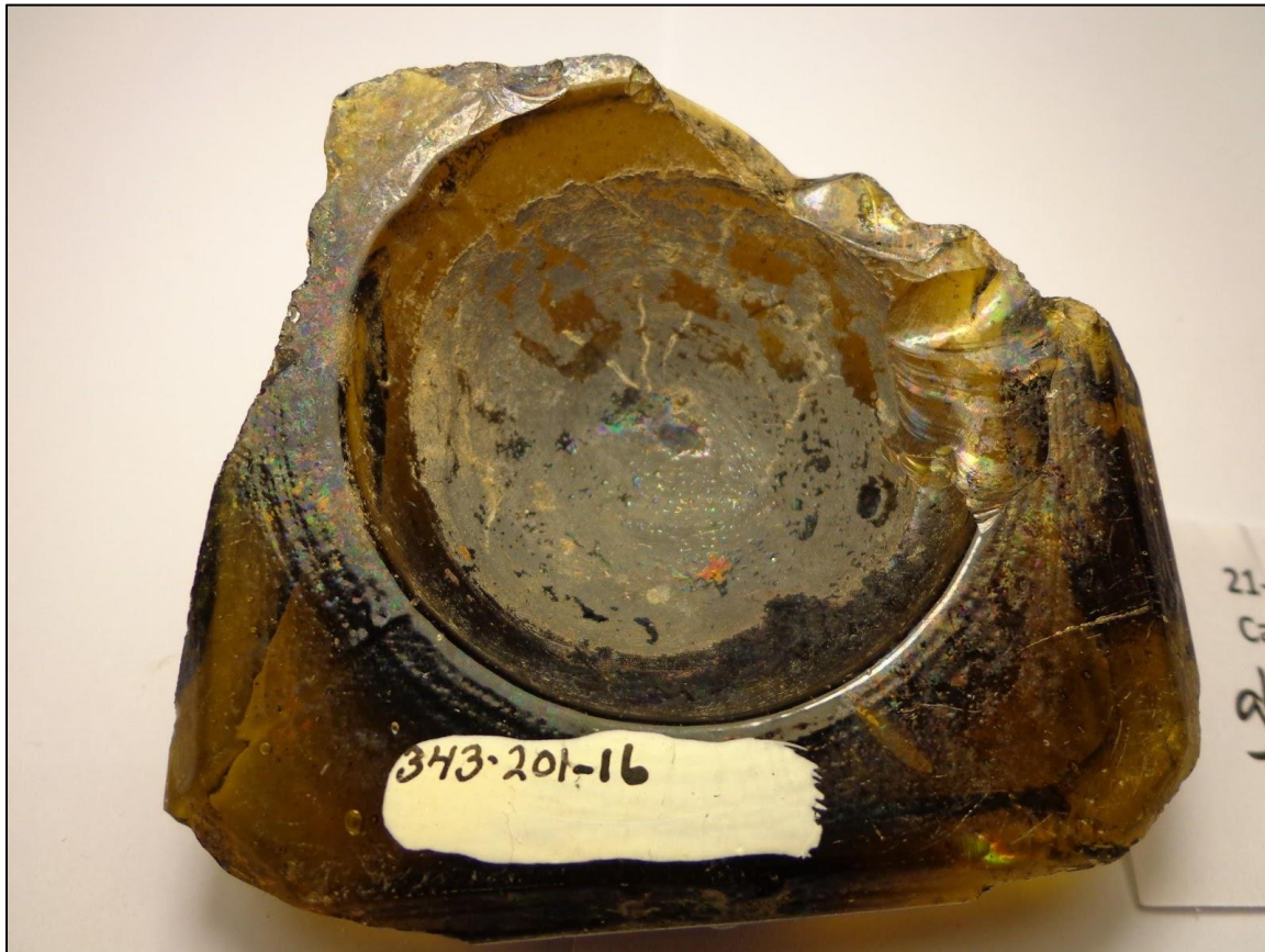
Figure 6: Square case gin bottle base, iron-tipped pontil scar visible. Long Barracks (Cat No 343.201.16).
