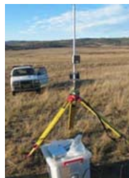
Fig. 2. Locata antenna (Barnes et al. 2005)
