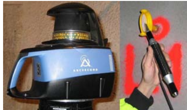
Fig. 5. iGPS transmitter and sensor during a test in a tunnel
