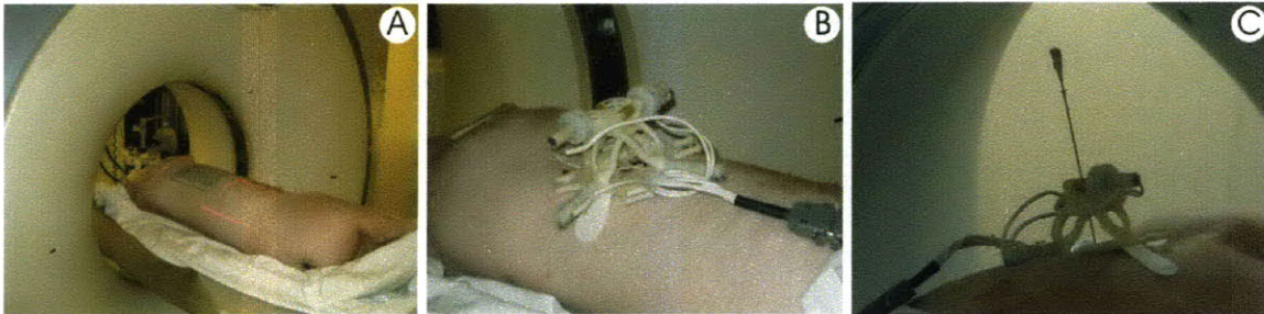
Figure 4-45 Porcine Testing. (A) Pig in scanner with targeting grid applied, (B) Device adhesive mounted to pig, (C) Needle orientation and insertion conducted remotely inside scanner.
