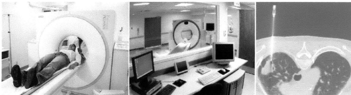
Figure 2-1 Left; a patient is shown lying on a CT scanner bed. Middle; the radiation shielded control room is shown where the physician would control the scanner and view the medical images. Right; a sample CT image is shown with a needle inserted into the lung.
