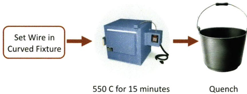
Figure 5-9 Illustration of heat-setting procedure for forming a shape in a thin piece of Nitinol wire.
