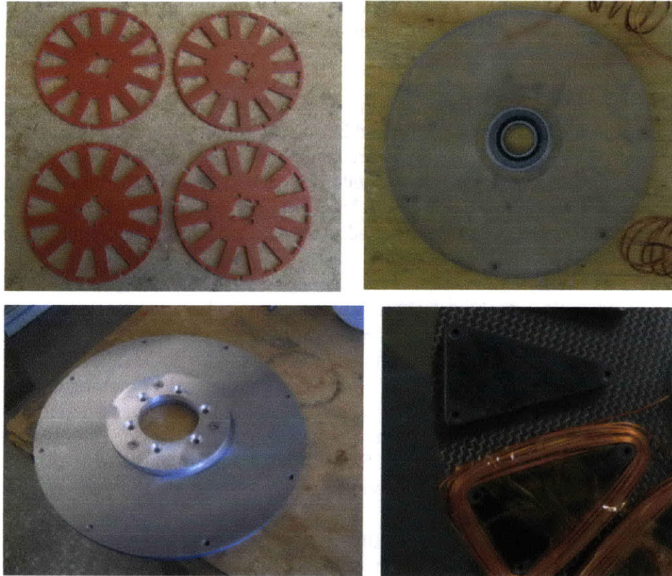
Figure 45: Part produced by abrasive water jet (with some finish machining): Insulating end laminations (top left), side plates (top right and bottom left), and winding inserts (bottom right).
