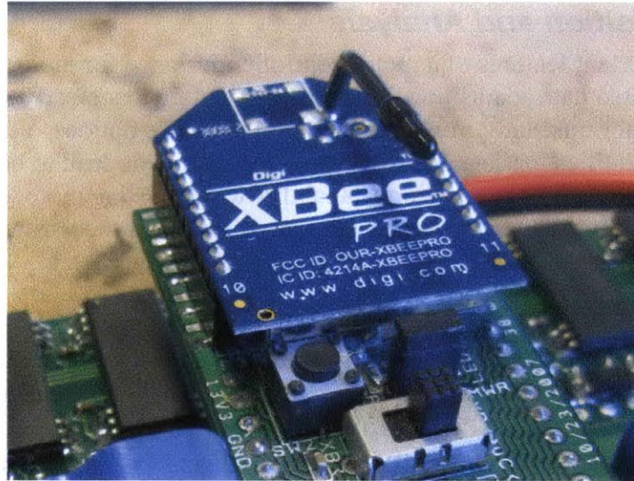
Figure 69: The 2.4GHz transceiver integrated into the case study motor controller.
