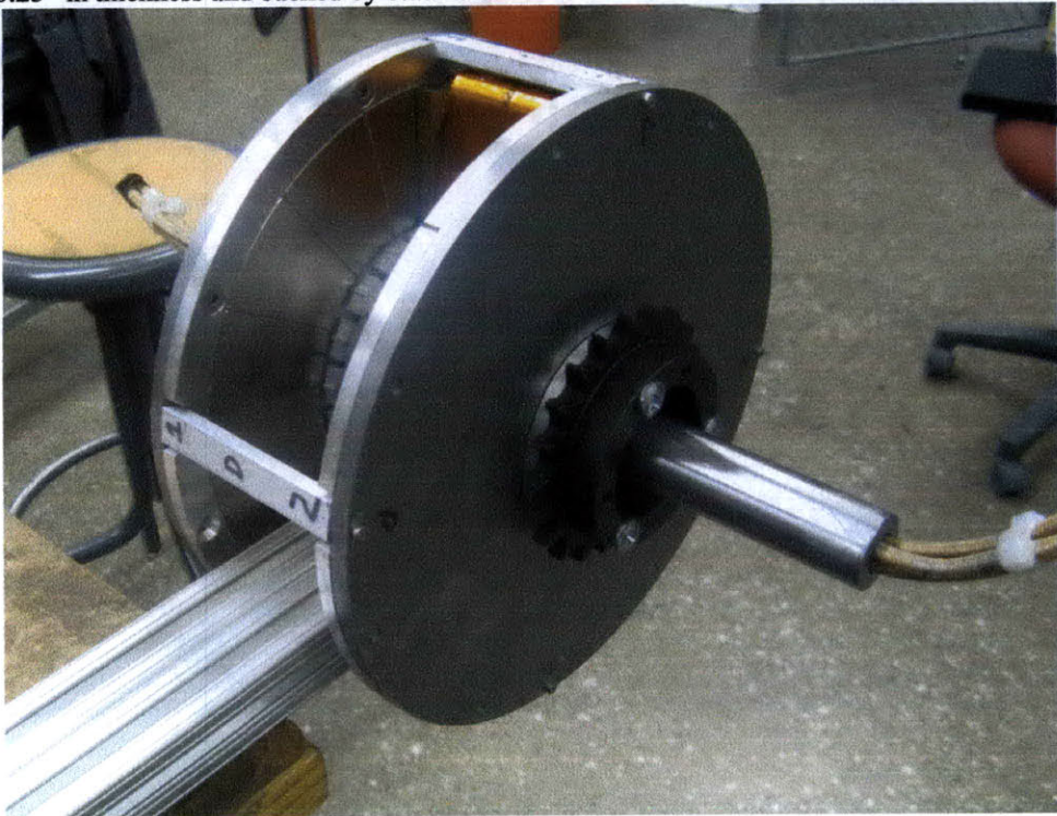
Figure 24: The assembled rotor disks and single stator segment for the original motor design of this case study.
