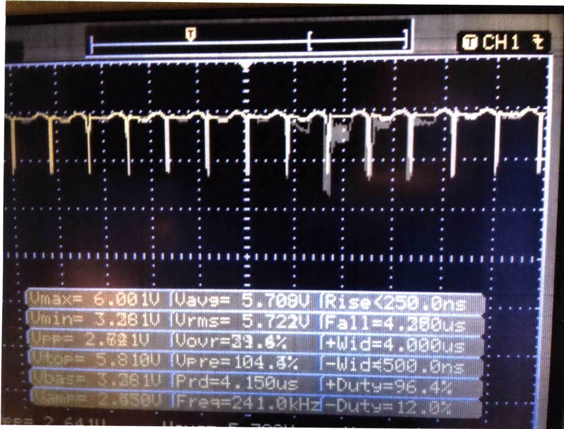
Figure 5: 300mF Supercapacitor Voltage Waveform Under Load Oscilloscope trace of super capacitor voltage during 130 Hz, 5 ms pulse width LED drive. 1 MHz peaking indicative of DC/DC converter switch operation.
