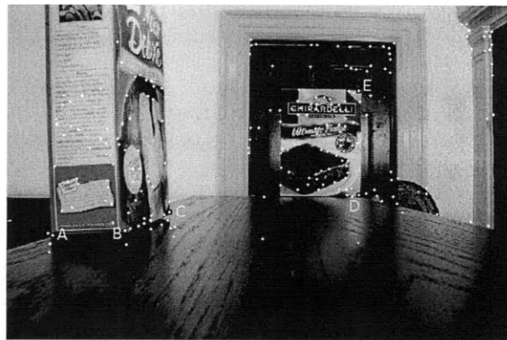
Figure 4-12: Single frame from cake box sequence. Feature points registered by Voodoo are marked with white dots. Selected feature points used for measurement are marked with white squares with black edges.
