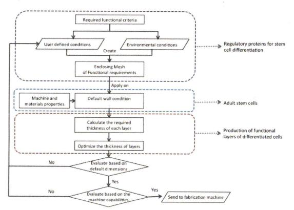
Figure 6.18. Form generation/ fabrication algorithm
