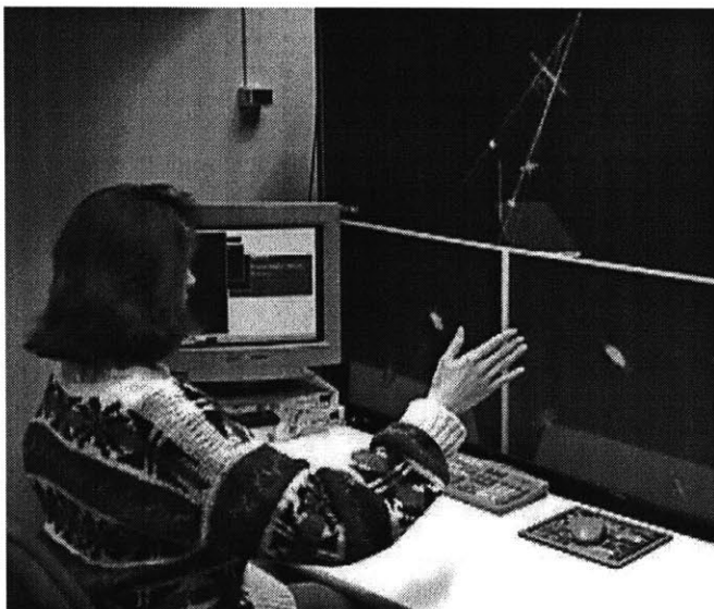
Figure 6-2: The Stereo Interactive Virtual Environment (STIVE) computer vision system used to collect data.
