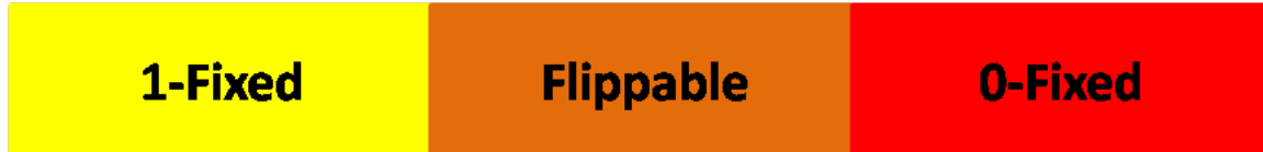
Figure 2-5: Division of devices into three categories based on their fall, rise, and flip timers. If a device is unable to move down, it is 1-fixed, and if it is unable to move up, it is 0-fixed. If it is neither, then it is flippable.
