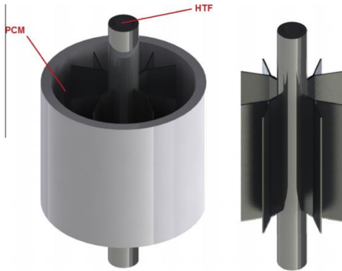
Figure 6 System analysed by Sciacovelli et al. [20], (HTF – heat transfer fluid)
