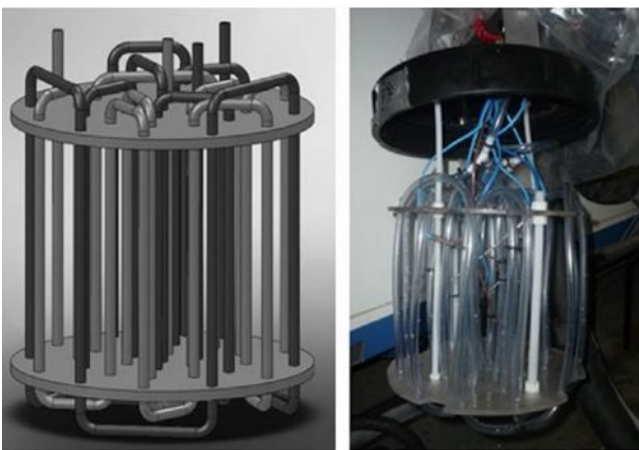
Figure 2 Schematic and photo of the experimental PCM tank with high heat transfer surface [17]
