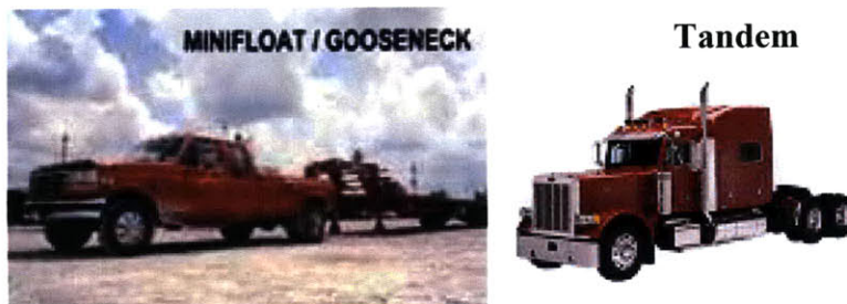
Figure 5. Minifloats can carry up to 15,000 lbs (~7 tools) and Tandem trucks can carry up to 45,000 lbs (~20 tools). The tandem is used exclusively for call outs where delivery time exceeds 11 hrs.
