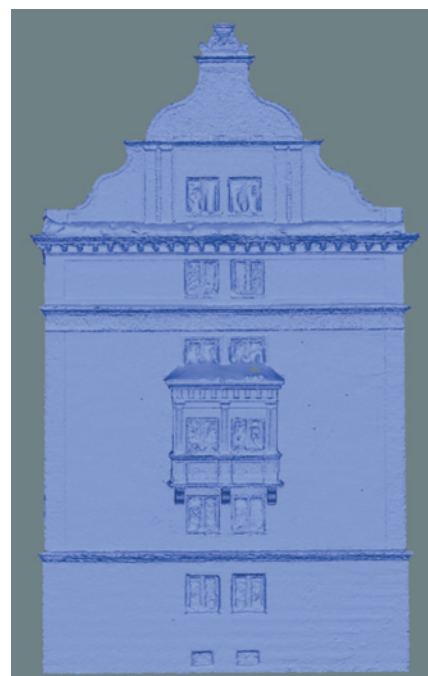
Fig. 9. 3D model of a residential building facade with poor texture
