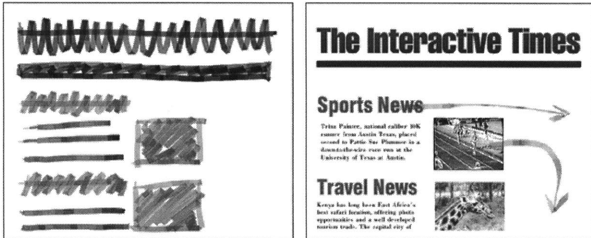
Figure 1.6: An example of how this system might be used to prototype the interface of an interactive newspaper or magazine. Sketched annotations at left are interpreted as canonical forms at right (we have added actual content for clarification) and sketched marks indicate how title title "Sports News" and the video clip associated with it should play out over time.
