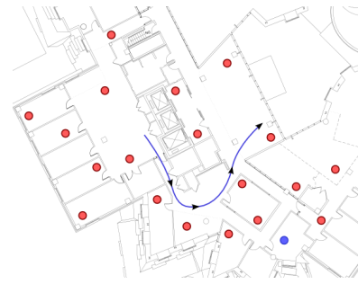
Fig. 6. Testbed. Dots refer to nodes; the line shows the path of the receiver in the mobility experiment when the blue dot was the transmitter.
