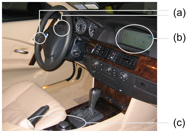
Figure 6-2: The interior control panel of the vehicle. (a) steering wheel buttons, (b) navigation display, and (c) center console iDrive and buttons.
