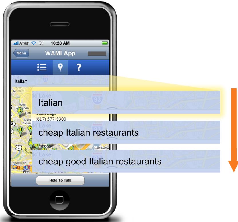
Figure 3-5: Streaming recognition results. As the user speaks to the system, the recognition results (shown in blue) are streamed immediately to the screen. Here the user is speaking, “Show me cheap Italian restaurants in Cambridge that are high quality.”
