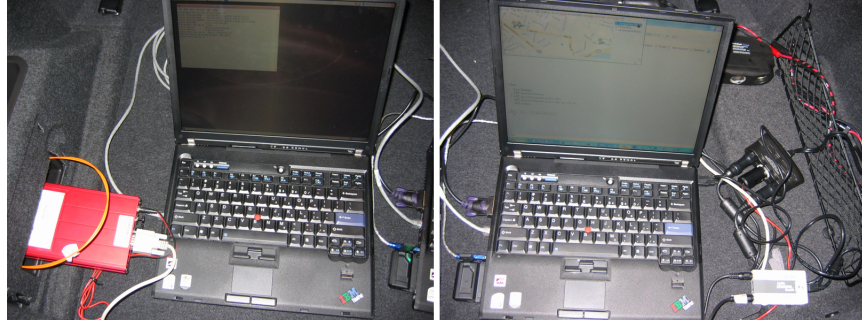
Figure 6-1: Vehicle System Configuration. One laptop acts as the language understanding processor, while the other interfaces with the vehicle.
