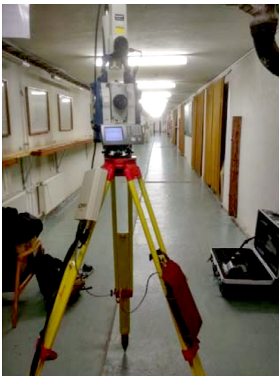
Figure 4. Determination of the device constant at the MMB
