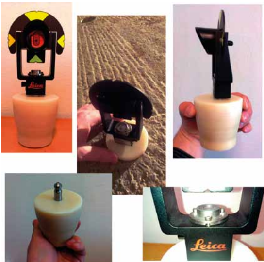
Fig. 2. Proposed truncated cone + Leica GPM 101 Professional
