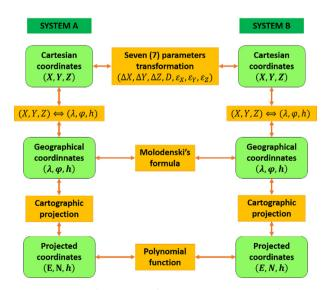
Fig. 1. Coordinates transformation process in geodesy (Dufour 2001)
