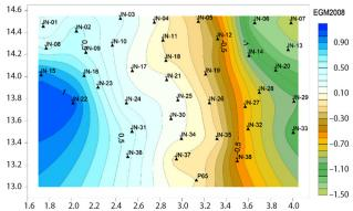
Fig. 7. Relative geoid of EGM2008 referenced to point no. 65
