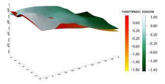
Fig. 11. 3D view of EGM2008 (green) and transformed geometric (red) geoids
