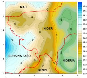
Fig. 5. Geoid Undulations from EGM2008 at d/o 2190. Source: Ibrahim Yahaya et al. 2017.
