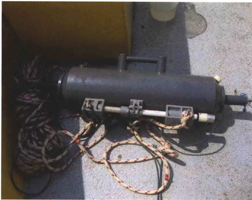
Figure 4.8 Niskin Water Sampler (AquaStore, 2005)
