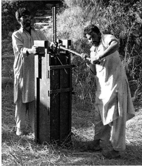
Figure 23: Local bale fabrication. Source: PAKSBAB “Straw Bale Fabrication”
