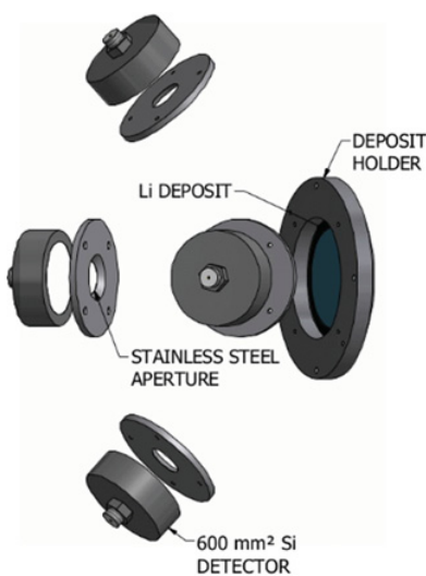
Figure 4. A representation of the layout of the flux monitor used in the BL2 experiment.
