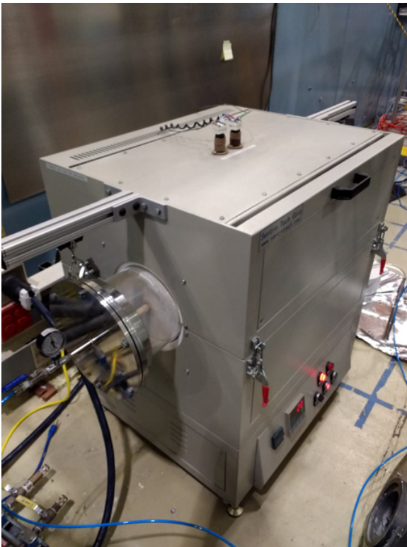
Figure 6. The large tube Furnace [14] used in the annealing work of Ref. [6].
