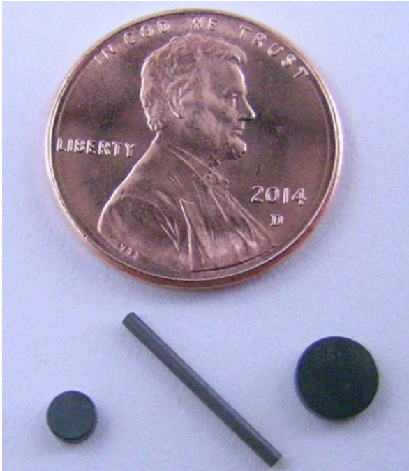
Fig. 1. SiC temperature monitors available for use in irradiation testing include small rods and discs. Only rods were used in this test. Monitors photographed with US cent for size perspective.
