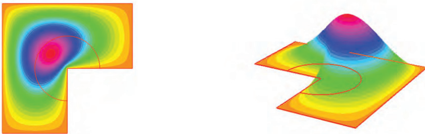
Figure 8. Stream function \psi in the whole domain \omega : 2-d view (left) and 3-d view (right).
