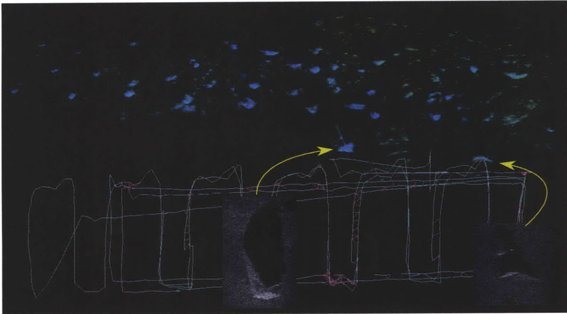
Figure 4-5: Sonar map of the MIT Sailing Pavilion. The map consists of all the features in the key frames used. The vehicle trajectory was smoothed using sonar frame registrations. The purple link show the loop closures that were used. The raw sonar images have been overlaid to better illustrate what the objects added to the map look like.
