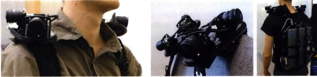
Figure 1-6: Our body-worn sensor suite includes four IEEE 1394 cameras mounted on the shoulders of the user, with a 360° field of view.
