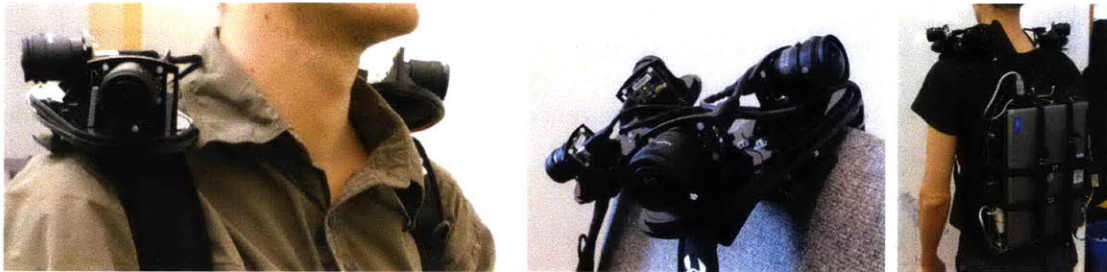
Figure 4-11: System overview including four cameras loosely mounted on the shoulder straps of a backpack. The horizontal field of view is 360^\circ . The system also incorporates a laptop, a 12V 4500mAh battery and a Firewire hub and can operate for three hours on a battery charge.
