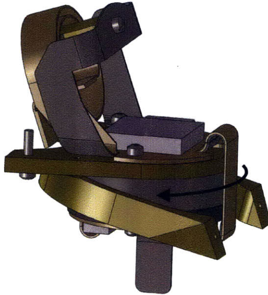
Figure 6-7: Millibot module. This assembly is repeated for each joint. The electropermanent stepper motor rotates the rotor joiner relative to the rest of the assembly, as shown. The rotor joiner connects to the processor bushing of its neighbor using two screws. See Figure 6-7 for an exploded view.
