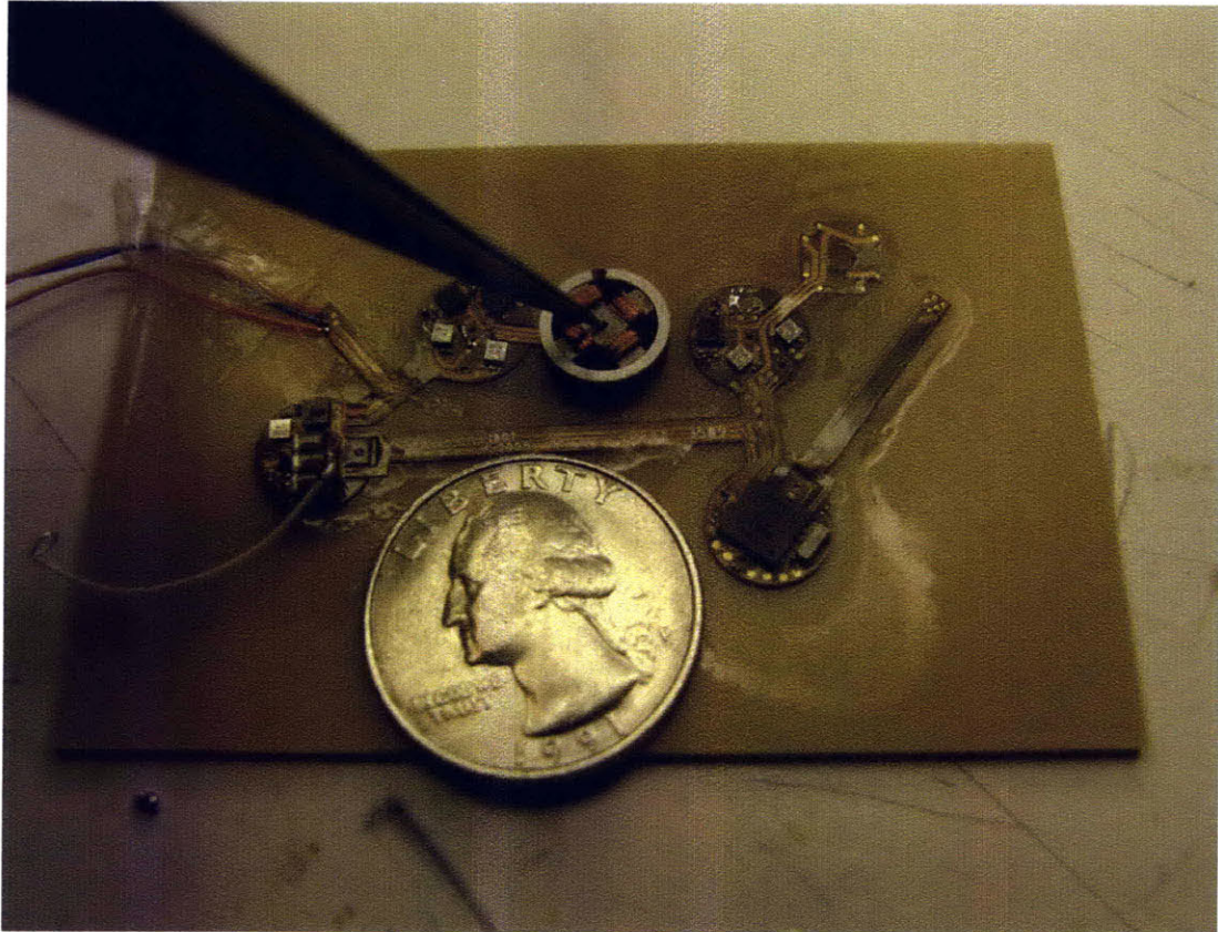
Figure 5-24: Complete friction-drive EP stepper, shown with an early version of the millibot flex circuit, which provides the drive pulses.
