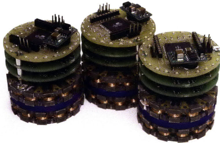
Figure 2-9: The planar magnetic Catoms. The cylindrical modules are 45 mm in diameter. They use an array of electromagnets for cooperative actuation and inductive power transfer and communicate using an array of infrared LED's. [52]
