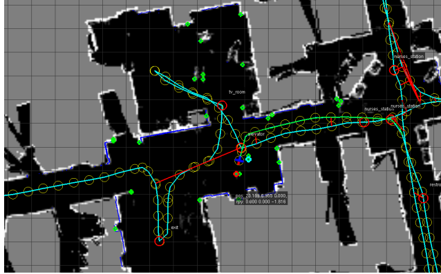
Figure 6-1: SLAM Output: Segments which might have been generated by legs are circled in green.
