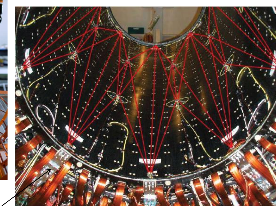
System consisting of 842 grid line interferometers, reference interferometer, and tunable laser for frequency scanning. The grid lines are arranged into geodetic grid, separate for the barrel and end-caps
