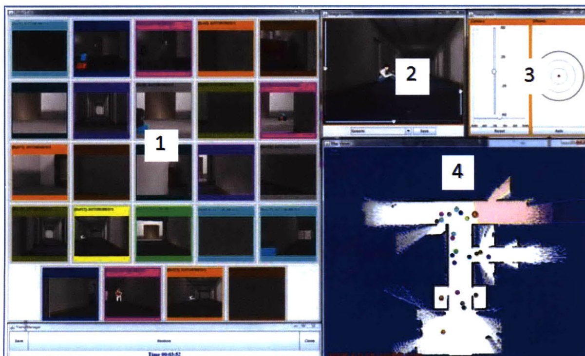
Figure 4.1 The MrCS interface with the four main sections numbered (1 Robot camera thumbnails, 2 Selected Robot camera view, 3 Robot control interface, 4 Map view) (Lewis, Wang et al. 2009).
