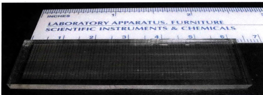
Figure 2 : Photograph of a PDMS microarray. Each microwell in 50 \mu m in diameter with the entire array comprising ~85,000 features.
